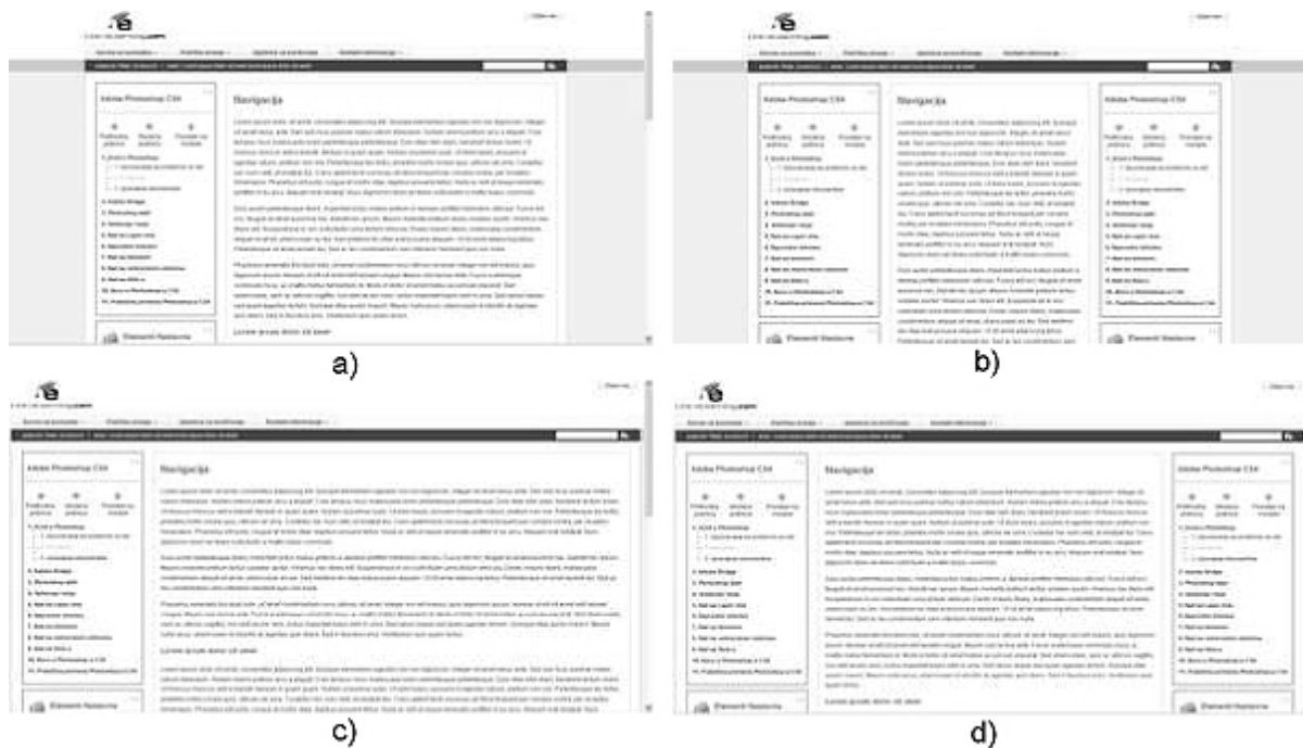
Figure 1. GUI template – a) normal width, one sidebar; b) normal width, two sidebars; c) full screen width, one sidebar; d) full screen width, two sidebars
